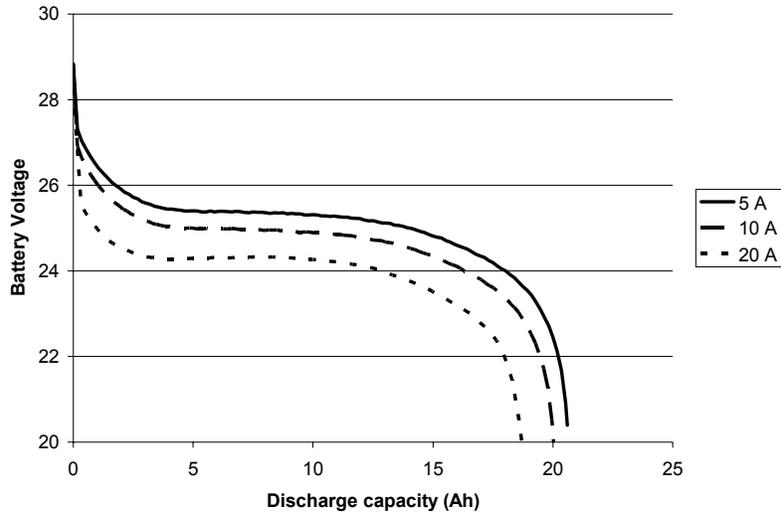
Figure 7: 500 Wh Module Discharge Characteristics
