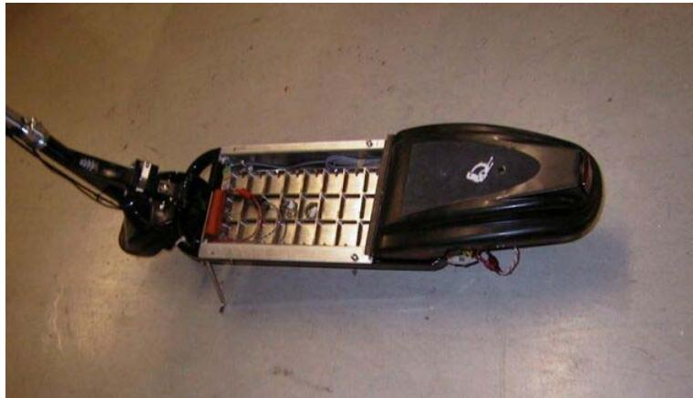
Figure 8: 24 Volt, 20 Ah batteries in electric scooter
