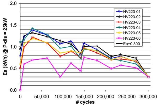
Figure 12. Energy fade rate for 6 Ah cell series
