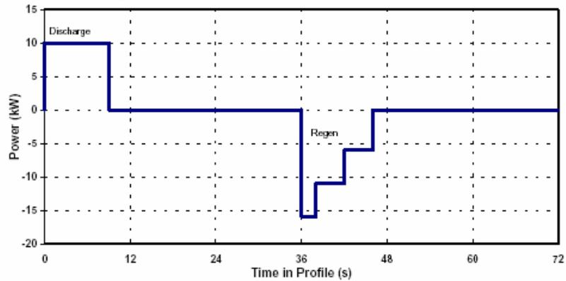
Figure 9. Power assist hybrid vehicle life cycle
