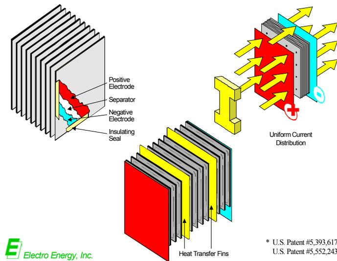
Figure 1: Schematic depiction of the wafer bipolar battery design
