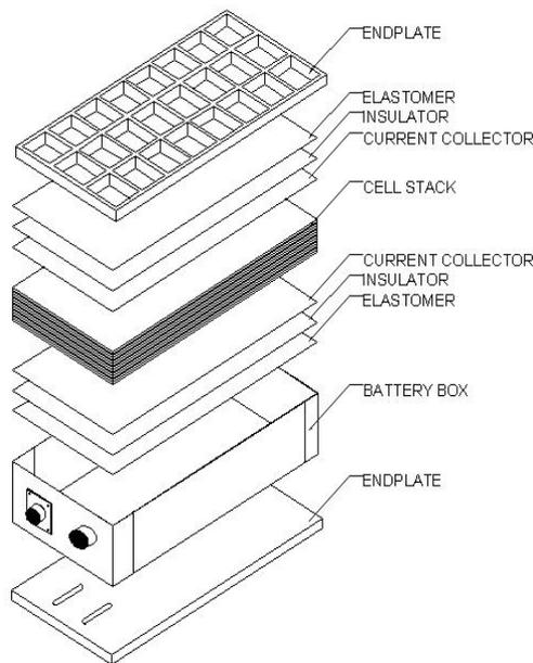
Figure 3: 20 Cell, 500 Wh Configuration
