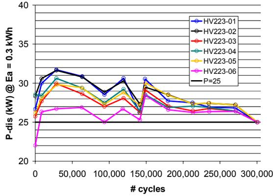
Figure 11. Power fade rate for 6 Ah cell series
