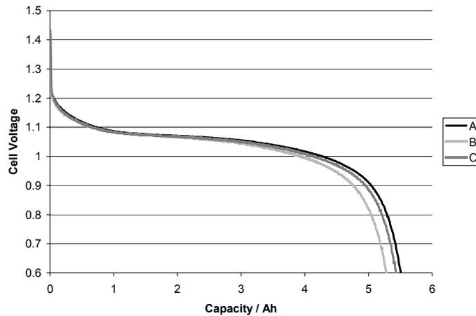
Figure 10. Discharge characteristics of 6 Ah cells at 80 amperes
