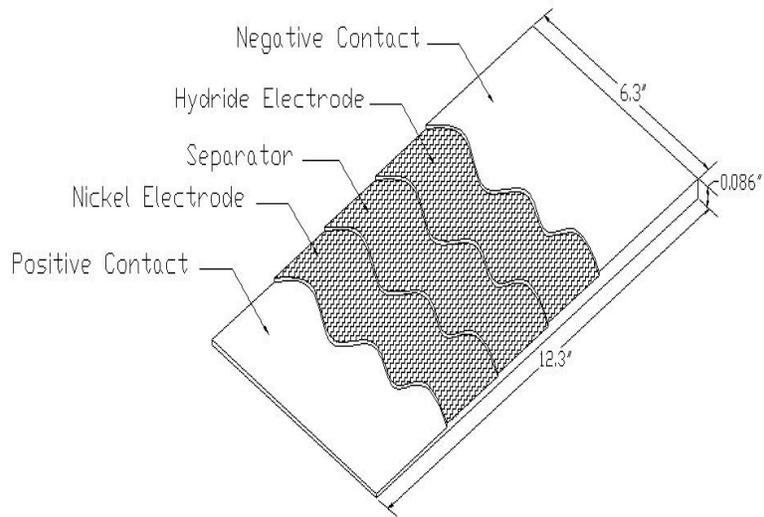
Figure 2: Typical cell layout
