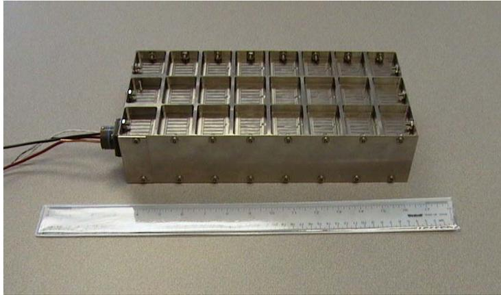
Figure 4: 24 Volt, 20 Ah Battery
